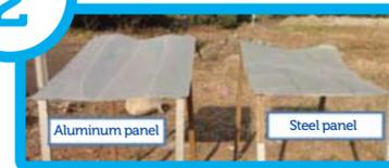
The temperatures of the upper and lower surfaces of each material were measured after one hour of exposure to direct sunlight
